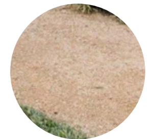
Crushed compacted gravel (Deco granite)
