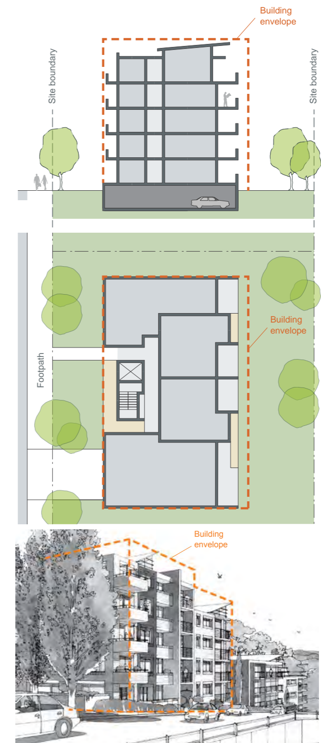
Figure 3.13: Apartment Design Guide - Loose fit envelopes
