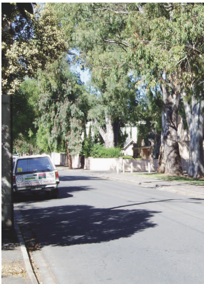
On-street parking should be provided on all streets – the design needs to respond to the type of street, number of lots accessed off the street and the character of the area. In this street the on-street parking is defined by the upright kerb as part of the carriageway with cars able to park on either side of the street.
