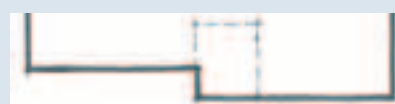
Slab design: front porch integral to house slab with minimal set down.
