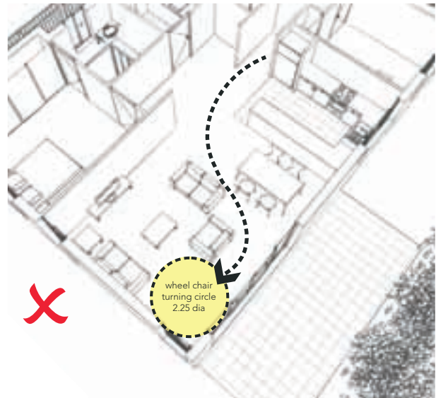
Turning space positioned in the far corner of the living room is illogical.
