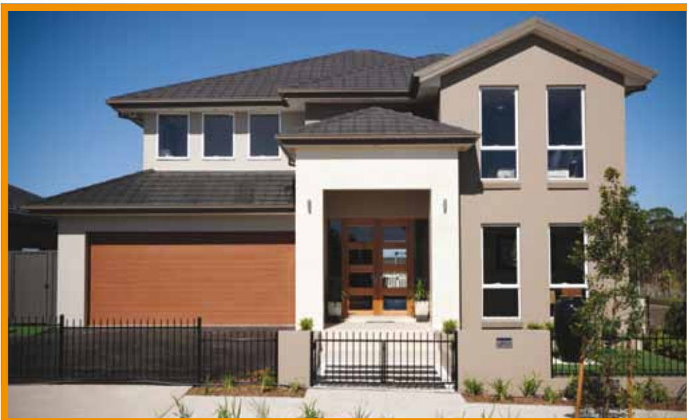
A black metal fence, 900mm high, is required on all lots on Steeltrap Drive or facing the Heritage Park. The fence incorporates the required plain, bagged brick letterbox pier.
